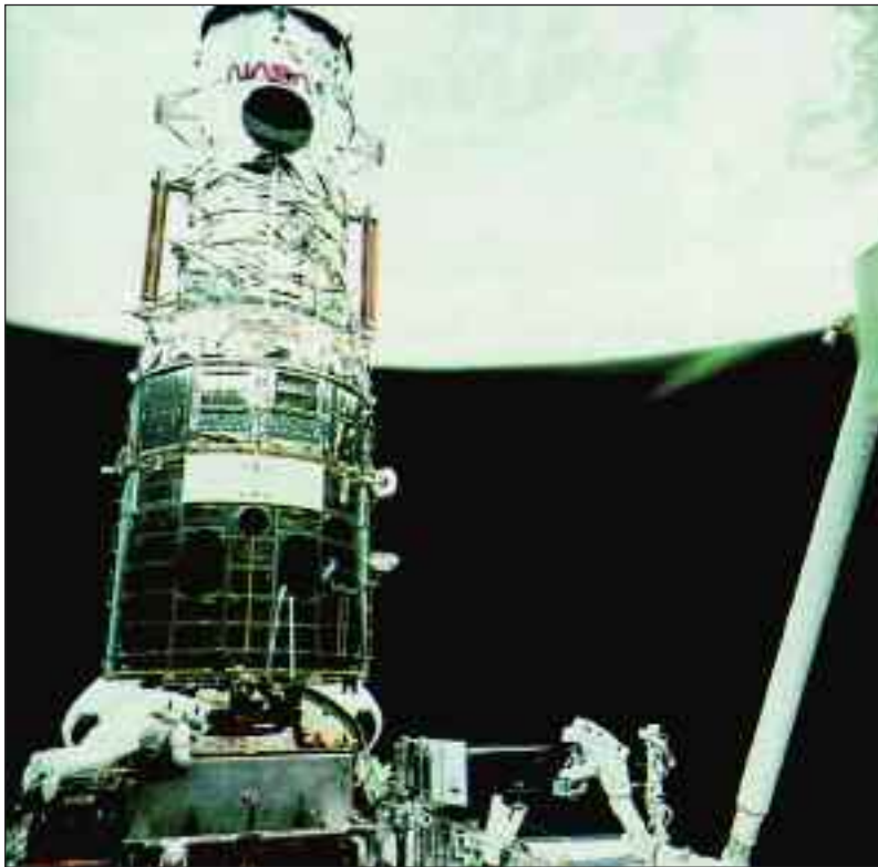
Two astronauts repairing and servicing the Hubble Space Telescope
