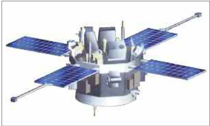
Image of the Helios spacecraft: designed to operate in an environment with extremely low temperature, extremely low pressure, and no aerodynamic drag
