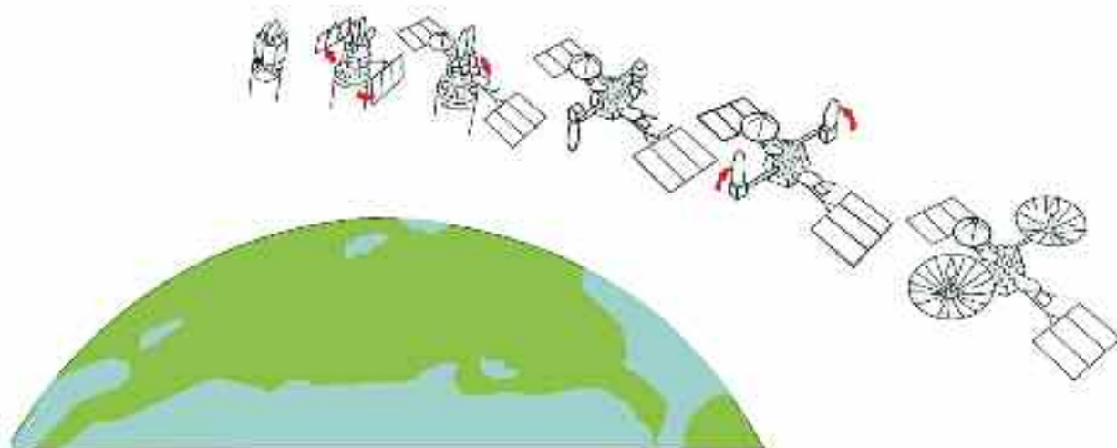
The Satellite unfolds until its antennas and solar panels stretch to dimensions larger than the size if a house.
