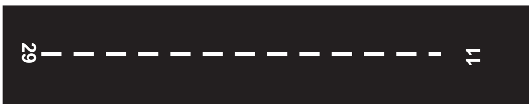
A typical VFR runway where the numbers "29" and "11" are based on magnetic headings of 290° and 110°
