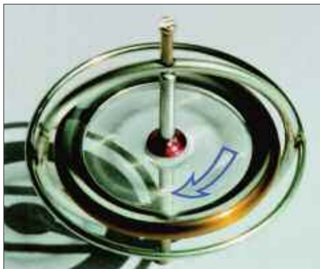
A toy gyroscope shows how it can maintain its position while spinning. When the rotor is spinning perpendicular to the surface, it is parallel to the horizon. The attitude indicator is based on this principle. It gives the pilot an “artificial horizon.”
