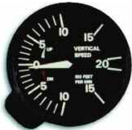
The vertical velocity indicator displays a rate of change in altitude
