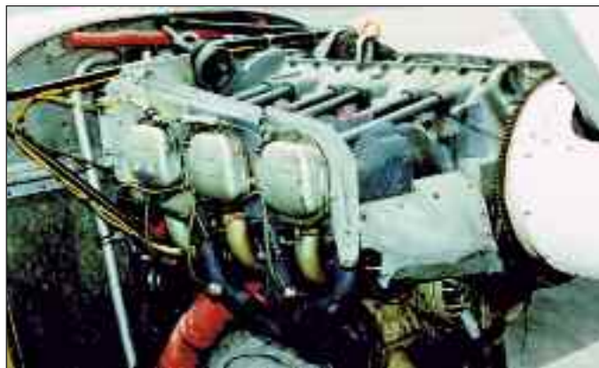
A horizontally opposed avco lycoming aircraft engine
