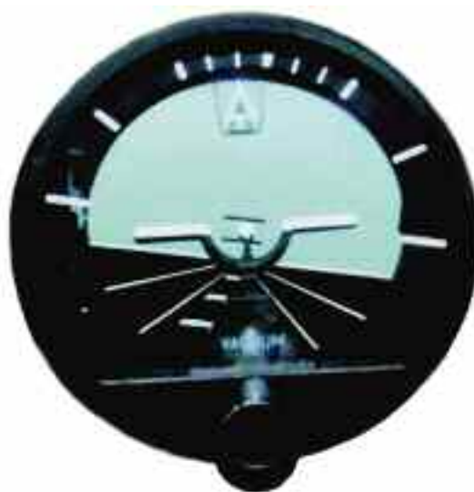
A toy gyroscope shows how it can maintain its position while spinning. When the rotor is spinning perpendicular to the surface, it is parallel to the horizon. The attitude indicator is based on this principle. It gives the pilot an “artificial horizon.”
