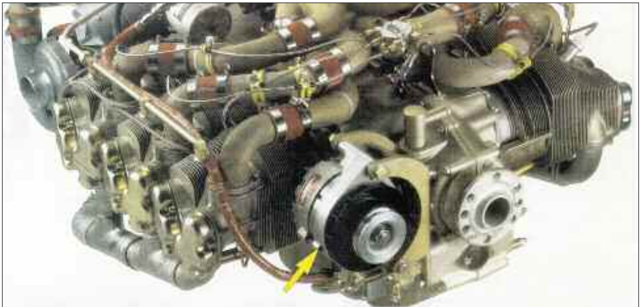
The alternator on an airplane engine looks much like the one on an automobile. Photo Courtesy of Teledyne Continental
